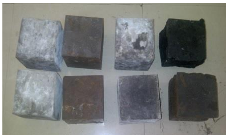
Fig 2: Geopolymer Concrete cubes size 150 x 150 x 150
