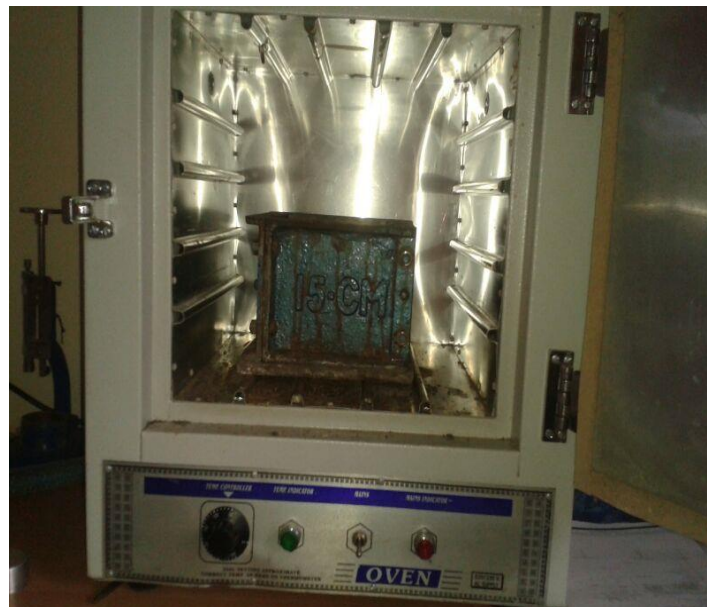
Fig 1: Oven curing of geopolymer concrete cubes at 60°C
